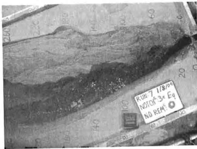
Figure 7-7. View of the original delta area in run 3xL at the static equilibrium following complete dam removal.
