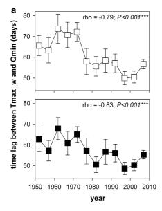
**Fig. 3** Time lag (as number of days) between annual hydroclimatic events. **a** Number of days that annual stream temperature maxima ( $T_{\text{max\_w}}$ ) preceded annual stream flow minima ( $Q_{\text{min}}$ ) for 1-d ( $open\ square$ ) and 7-d MA ( $filled\ square$ ) events. **b** Number of days that annual stream temperature maxima ( $T_{\text{max\_w}}$ ) preceded annual air temperature maxima
