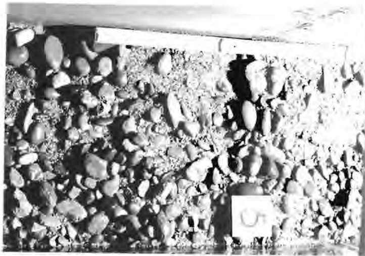
Figure 4: An example of a step-pool. Note the imbricated particles in the step and fines filling the downstream area (pool). Flow is from right to left. Scale is graduated in centimeters.
