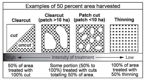
Figure 3—Forest harvest treatments that result in a reported value of 50 percent of area harvested. Theoretical intensity of treatment and predicted influence on peak flow changes decreases from left to right.
