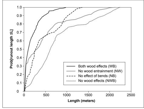
Runout length distributions simulated by the physics-based debris flow model, with and without wood.
