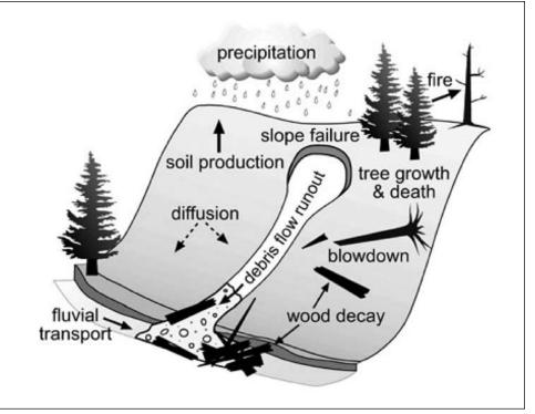
Many processes are involved in debris flows and must be incorporated into the simulation models.
